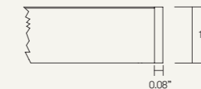
Edge Detail # 69 HPL laminate over a 1" MDF core with matching or solid PVC edge.
