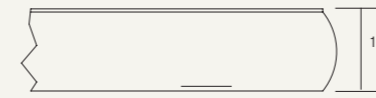
Edge Detail # 11 1" MDF core, specified laminate face and counterbalance with convex edge, as standard. The edge is clear finished as standard or can be stained.
